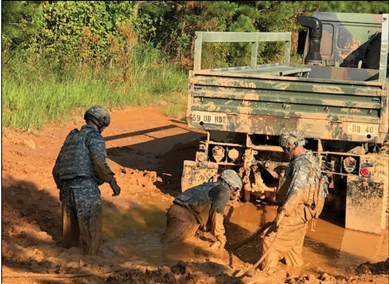
Figure 2-5. Recovery of a Mire Factor 2 MTV.
