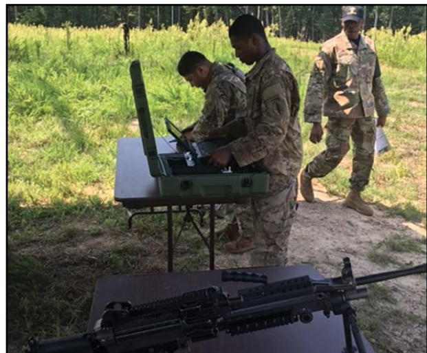
Figure 6-2. Using an MSD to troubleshoot a weapon.
