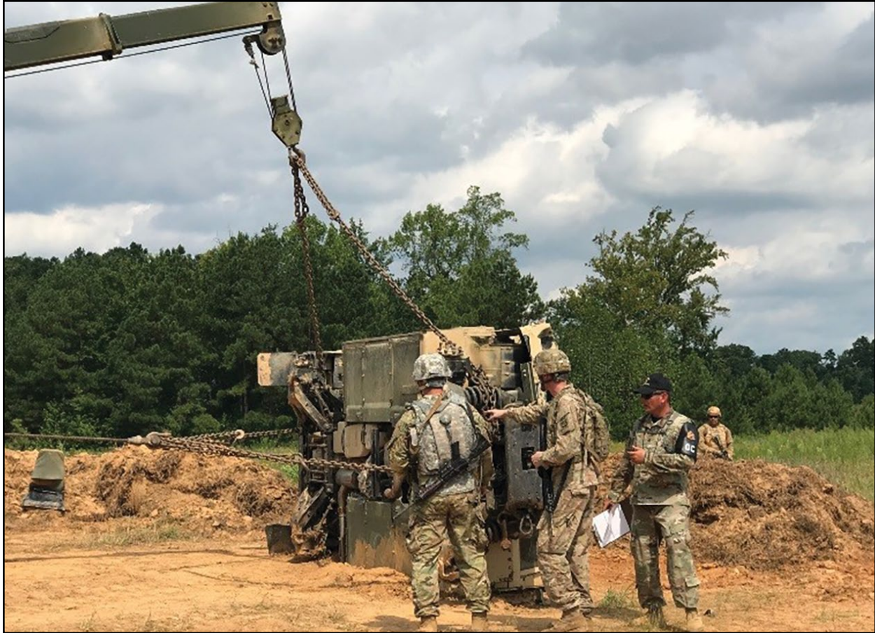
Figure 2-2. An evaluator inspects the proper rigging procedures for recovering an overturned vehicle.
