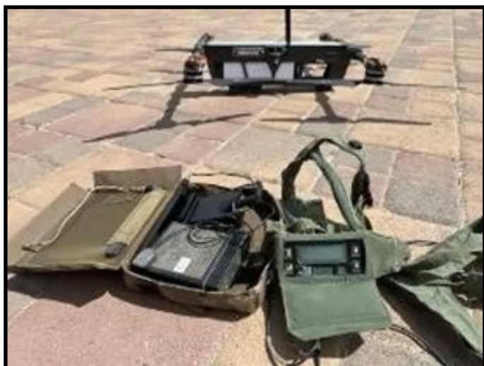
Soldier Instrumentable- Multiple Integrated Laser Engagement System (I-MILES) and a TS-M800 Block 3 drone.
