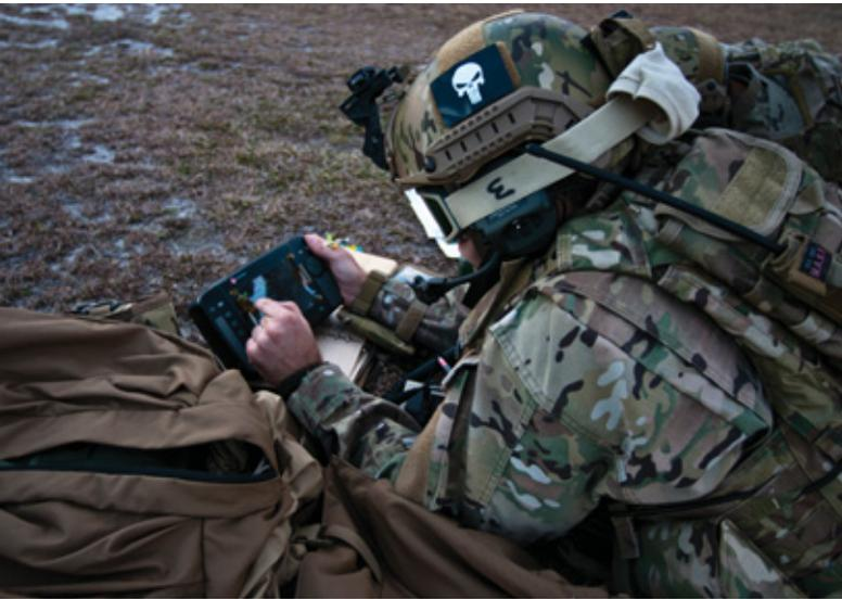
U.S. Air Force SrA Sean Almond, tactical air control party with the 147th Air Support Operations Squadron, Texas Air National Guard, uses a ROVER 5 handheld portable transceiver device to view targeting data while performing close air support training at the Townsend Bombing Range during exercise Global Guardian, McIntosh County, GA, 16 February 2012. (U.S. Air Force, SSgt Jorge Intriago)
