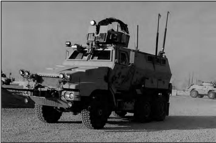
Figure 18. Mine-Resistant Ambush Protected (MRAP) Vehicle.
